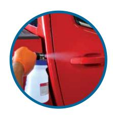
Misting is used predominately for the application of disinfectants. The misting equipment generates a mist or fog formed of Ultra Low Volume (ULV) droplets. Through vaporization, airborne and surface-based pathogens are destroyed, so there is no need to move furniture or equipment around for the treatment to work.
